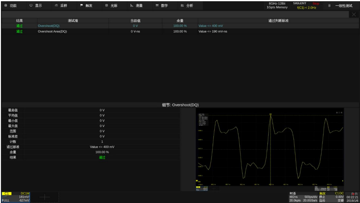
图 11.27-4 DDR3 Overshoot(DQ)和 Overshoot Area(DQ)测试示例
