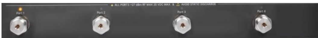
Figure 5-7 Front panel RF connectors (4-port VNA)
