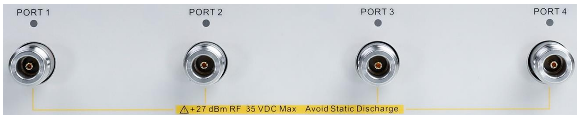
Figure 5-6 Front panel RF connectors (4-port VNA)
