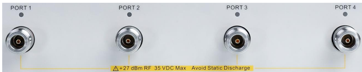
Figure 5-6 Front panel RF connectors (4-port VNA)
