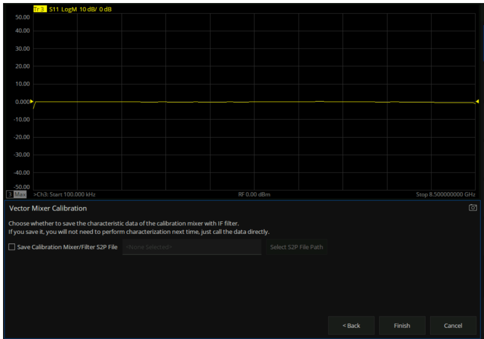
Characterization and calibration of mixer/filter combination, save S2P interface
