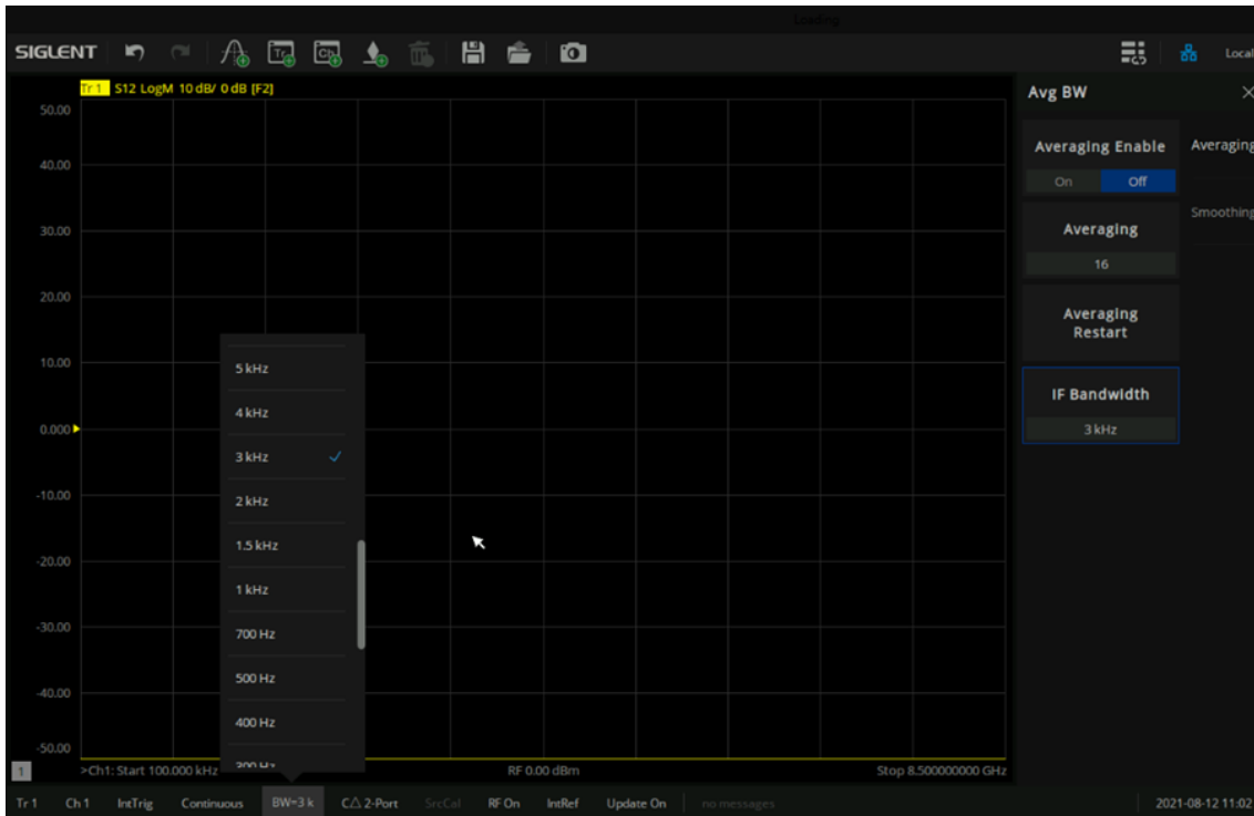
Figure 6-9 Set the IF from the status bar
