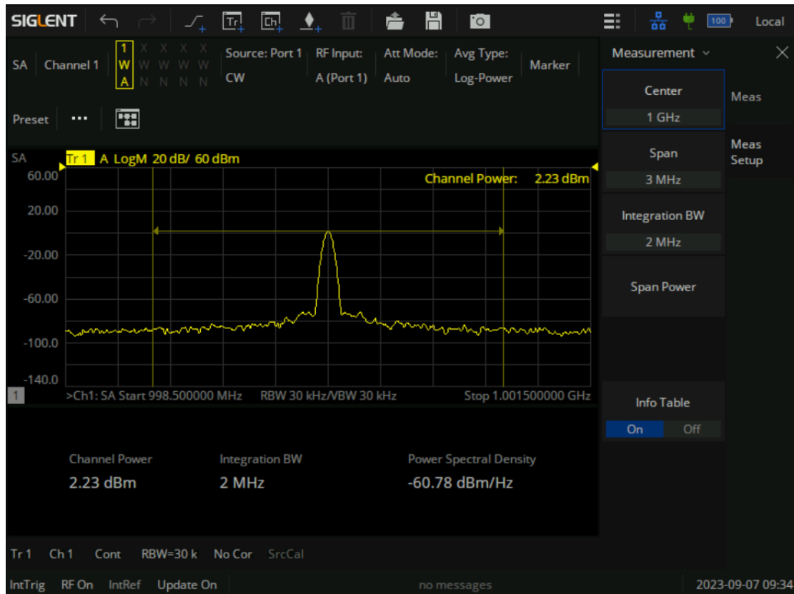
Figure 11-12 Channel Power measure
