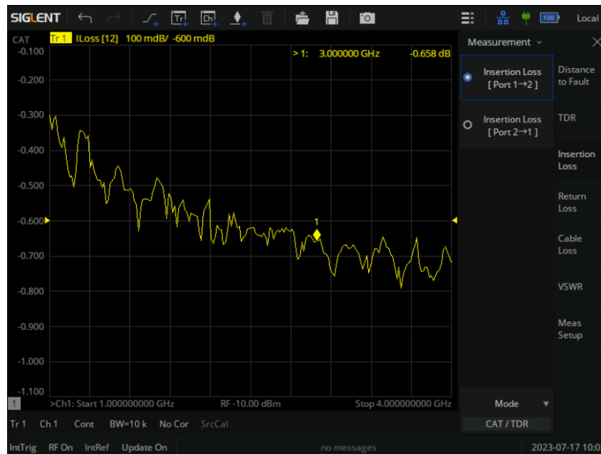
Figure 13-6 Insertion loss measurement interface
