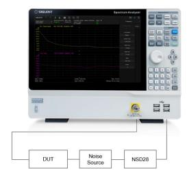
Since the noise source operates on 28V DC and requires switching between high (hot) and low (cold) states during testing, SIGLENT provides the NSD28 Noise Source Driver Module. The SSA5000-NF Noise Figure application controls this module via USB to automatically implement switching control.
