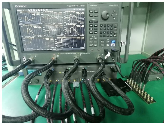
Figure1: Siglent Vector Network Analyzer SNA6000 Series equipped with SSM5000A Switch Matrix enabling 24-port expansion
