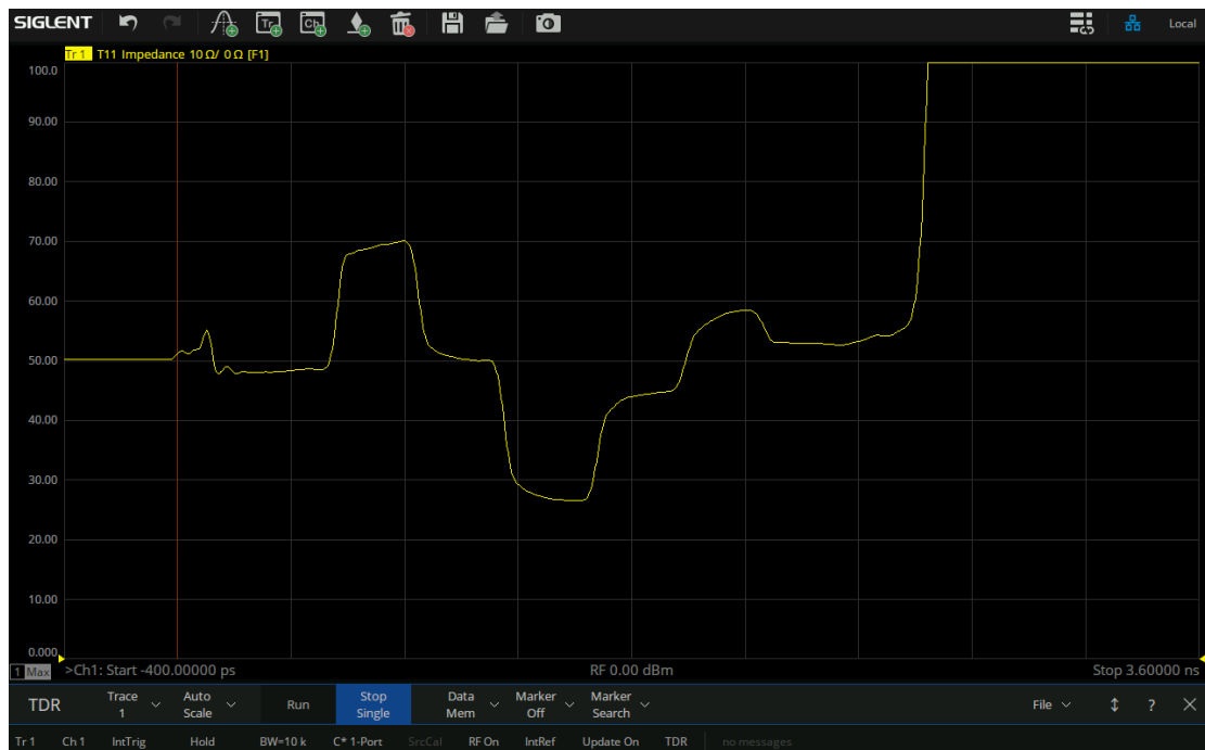
Figure 5: Characteristic impedance testing in TDA mode
