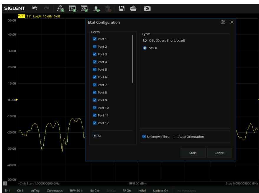
Figure 2: Calibration wizard for multi-port electronic calibration module
