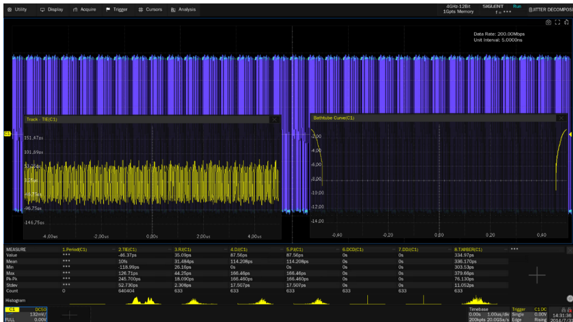
Figure 3.4 Jitter Analysis Using SDS7000A
