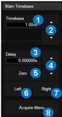
1. Set the horizontal scale (timebase) by the virtual keypad
