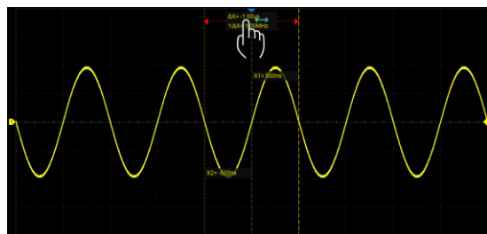
Touch and drag the cursor information region to move the pair of cursors simultaneously
