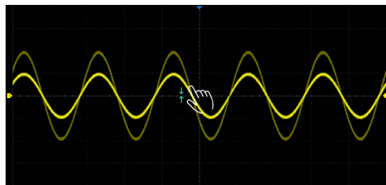
Pinch and spread the waveform vertically to re-scale the vertical gain
