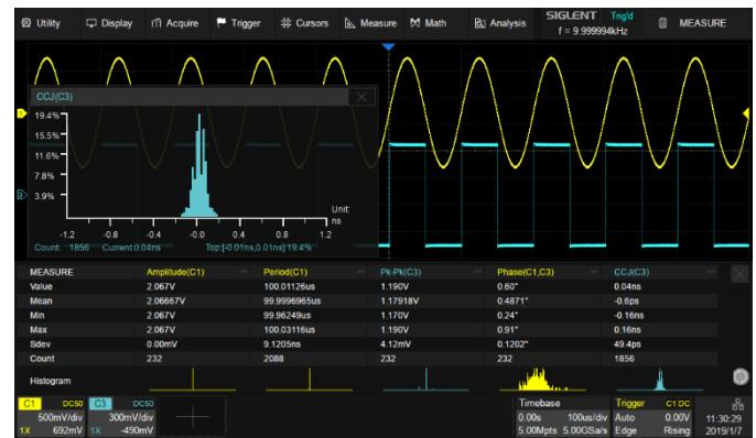
Statistics shows the current value, maximum value, minimum value, standard deviation and mean value of up to 12 parameters simultaneously. Histogram is available to show the probability distribution of a parameter. Trend is available to show the parameter value vs. time
