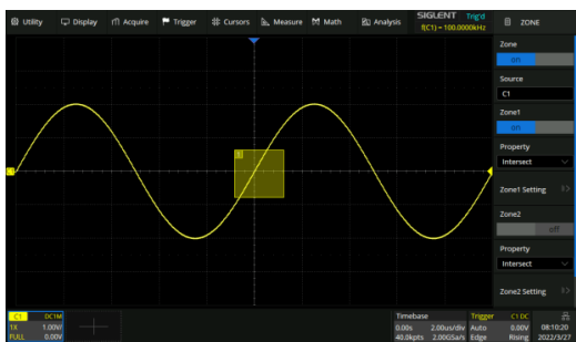
Select C1 as the source, turn on zone1, and set the property as "Intersect"
