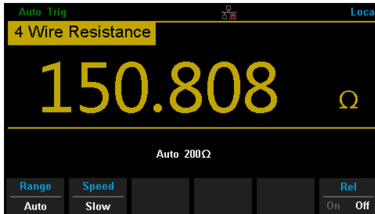
Diagram 2-15 4-Wire Resistance Measurement Interface
