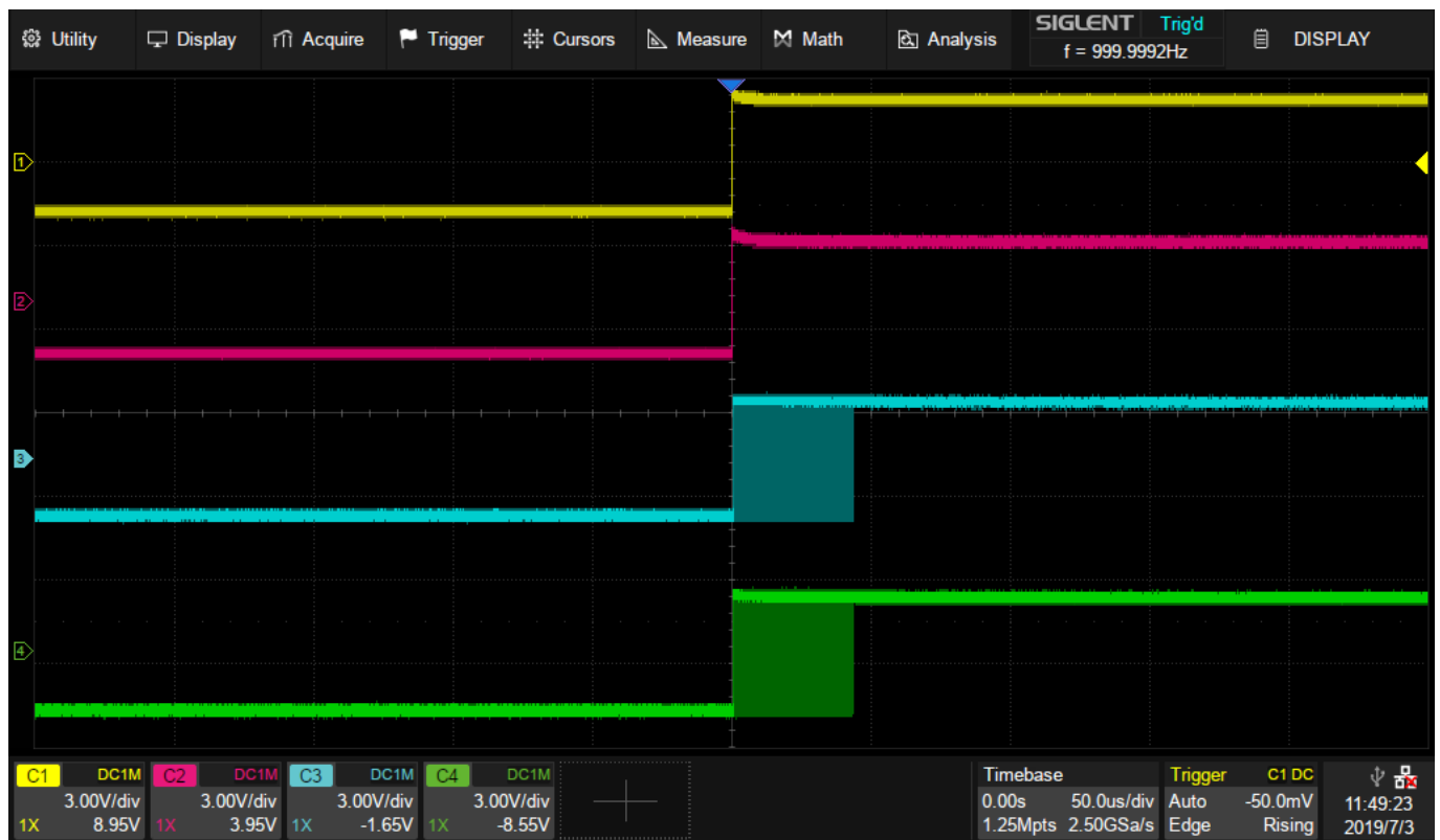
Figure 4. Four signals phase drift without synchronization
