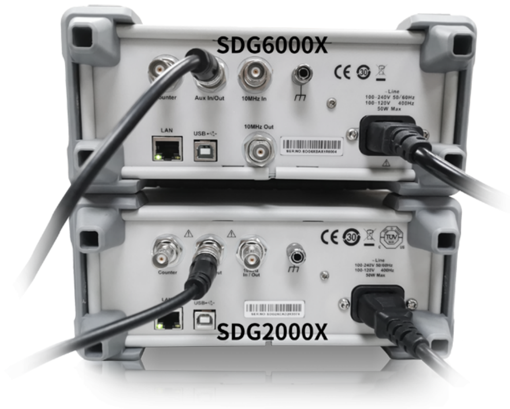
Figure 2. Connect SDG2000X and SDG6000X Aux In/Out
